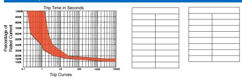
Breaker must hold 100% of rated current and must trip at 150% and above, within the time limits shown in curve. Trip times specified at 25° ambient with no preloading.
